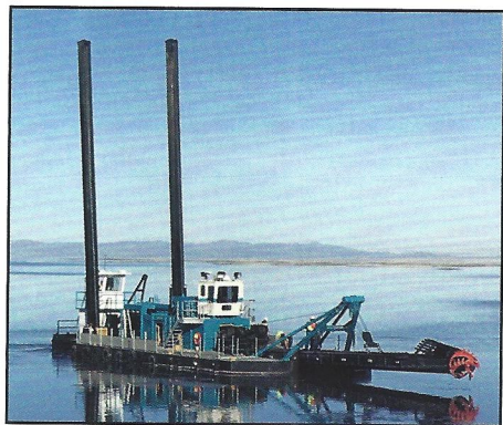
DSC Dredge Shark Class Dredge with first ever Tier 4 Final C32 ACERT Caterpillar engine.
