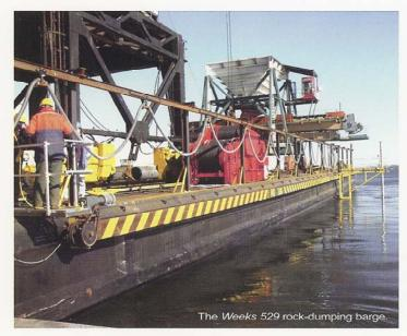
Weeks Marine (Cranford, NJ) was entrusted with one of the trickiest portions of the project – dumping rock over the installed pipeline in order to ensure it was protected against anchor dragging, etc. Proving the correct rock coverage had been met was essential not only from a design perspective, but also from a permitting stance. Weeks Marine was faced with four major obstacles:
