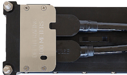
Figure 9: Seated connectors (Sonic 2024 on left and Sonic 2022 on right)
