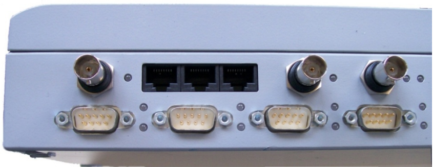
Figure 21: SIM Interfacing Physical Connections
