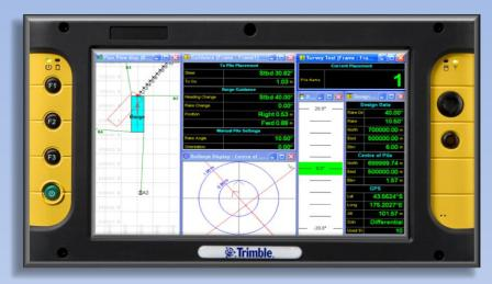
**Productivity.** Knowing the precise location and orientation of your rigs saves time in positioning the lead for each shaft or pile target. The rig operator is provided a real time display, information, and instructions to guide and position the rig to the next target. Final position of each target can be saved to "as-built" reports along with achieved accuracy metrics (actual vs. design).
